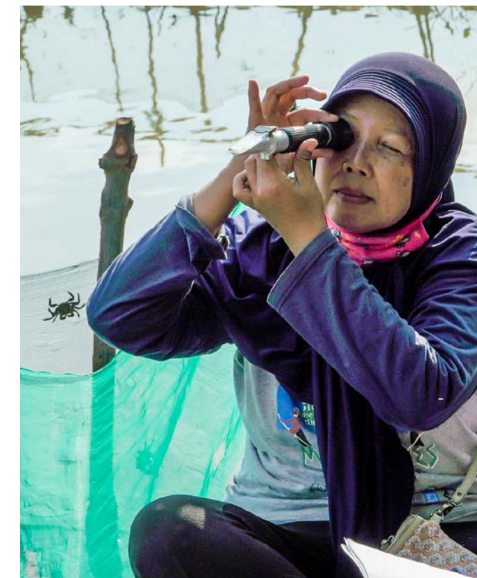
Local community use a refractometer to measure the salinity of the water, Indonesia.
