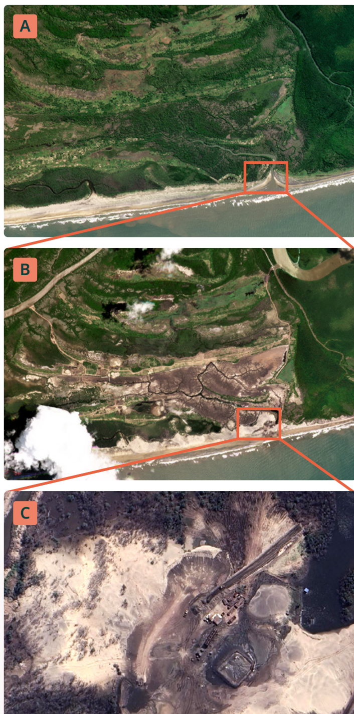
Figure 14. Illustrates the impact of the hydrological disturbance from sand mining, which blocked off the river channel and caused significant mangrove dieback. A) Planet NICFI Imagery from May 2022, before the disturbance; B) Planet NICFI imagery from February 2026, showing the impact of the sand mining. The red rectangle illustrates the location of the channel blockage. C) A very high resolution satellite image from Google Earth of the channel blockage showing the machinery and sand excavations.
