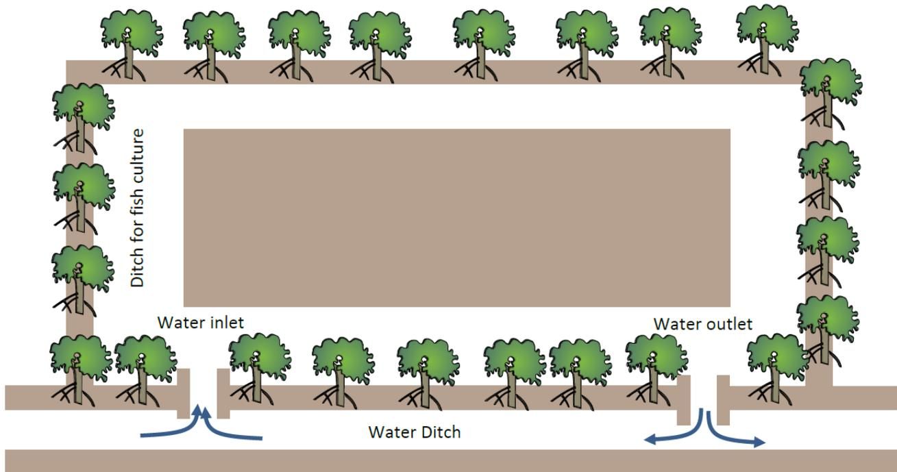
Model 7 (Type 2): Kao-Kao model with three separate ditches one-gate water inlet system. The water can flow from ditch to ditch, depending on tide (Sofiawan, 2000). Note that the lighter coloured areas are channels, not dykes. Illustrations by Audrie Siahainenia.
