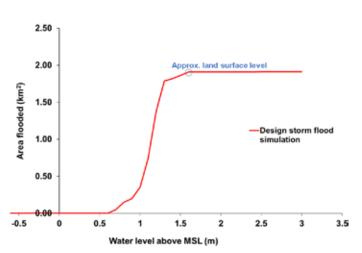
Figure 6. Area of land flooded on Hulhumalé against elevation above mean sea-level
