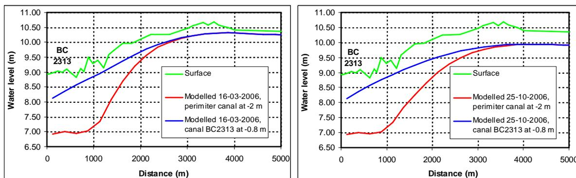
Figure 8 Modelled water depths for the dry year of 2006 (left: wet conditions; right: dry conditions), in the conservation area and in the buffer zone, for the hypothetical cases that A) the water level in the perimeter canal would be at 2m depth, or B) that the perimeter canal and drains in the buffer zone are fully closed and water depth water table in canal BC 2313 are kept at 0.8m depth.
