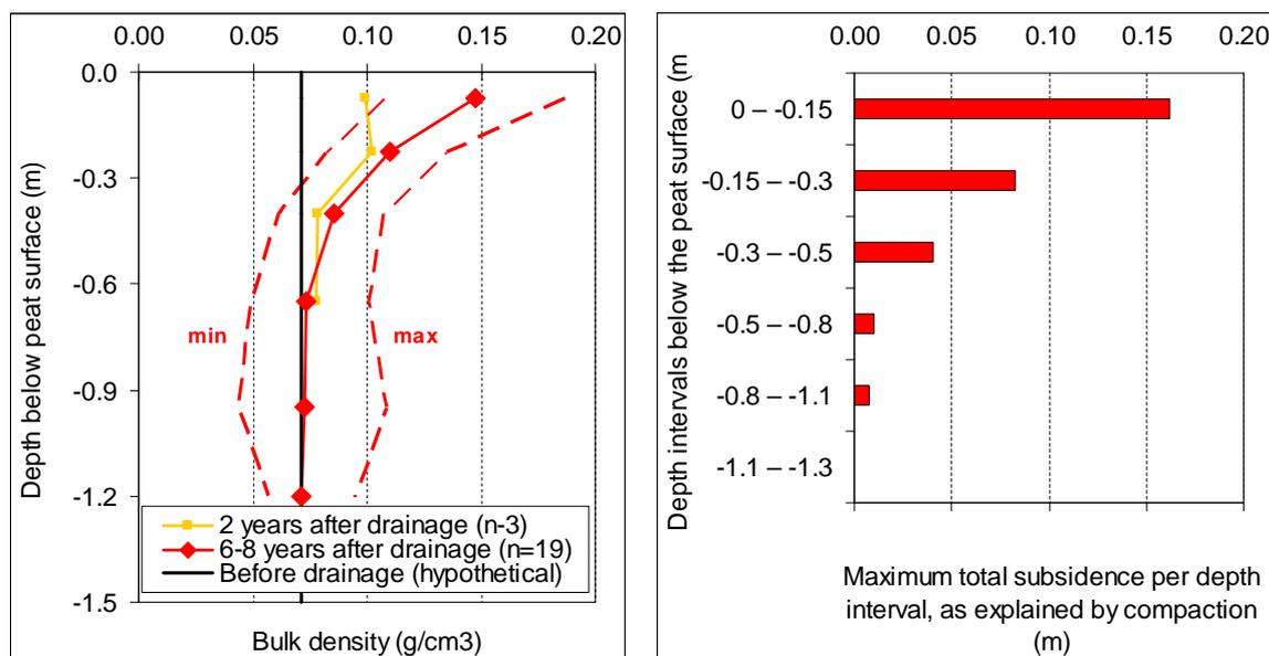
Figure 14 Preliminary analysis of Bulk Density data in Pelalawan plantations (left), and how much of total subsidence they may explain assuming an original BD of 0.07 g/cm (right). Bulk density samples were taken from the side of 22 soil pits that were dug to just below the water table in peat that is mostly fibric. Three replicate samples were taken at each standard depth; average values for each depth are presented here.
