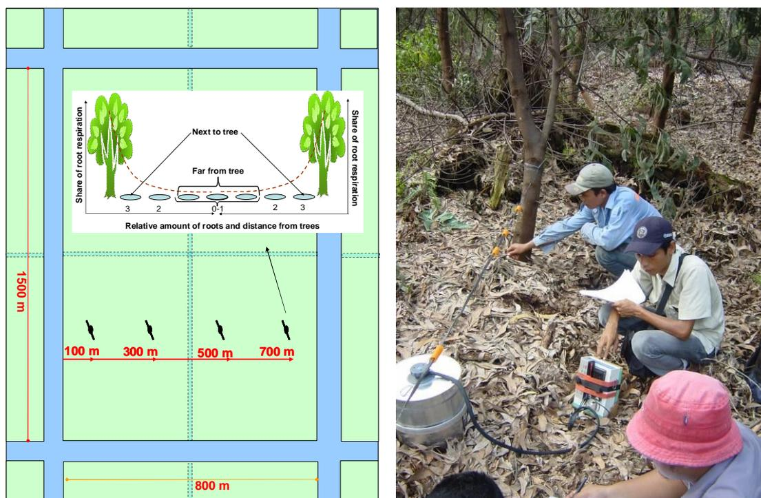
Figure 9 Schematic set-up of peat surface carbon gas emission measurement transect and sub-sites at compartment (on left), and CO<sub>2</sub>-flux monitoring event by EGM-4 infra red gas analyzer in progress (on right).
