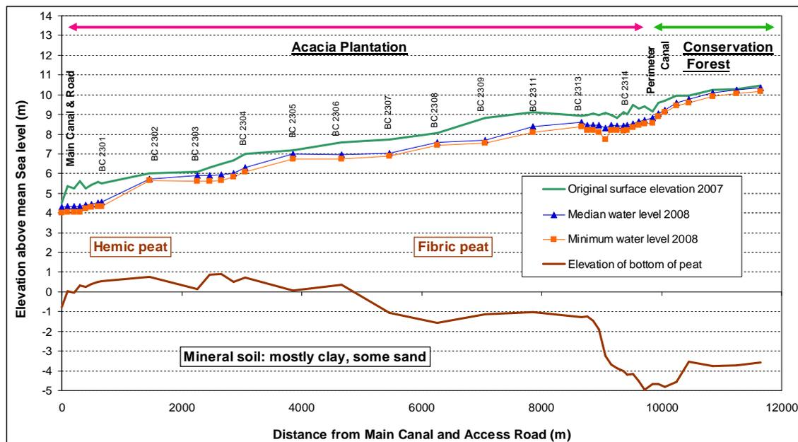
Figure 2 Cross section along the dipwell transect in the Phase 2 Pilot area.
