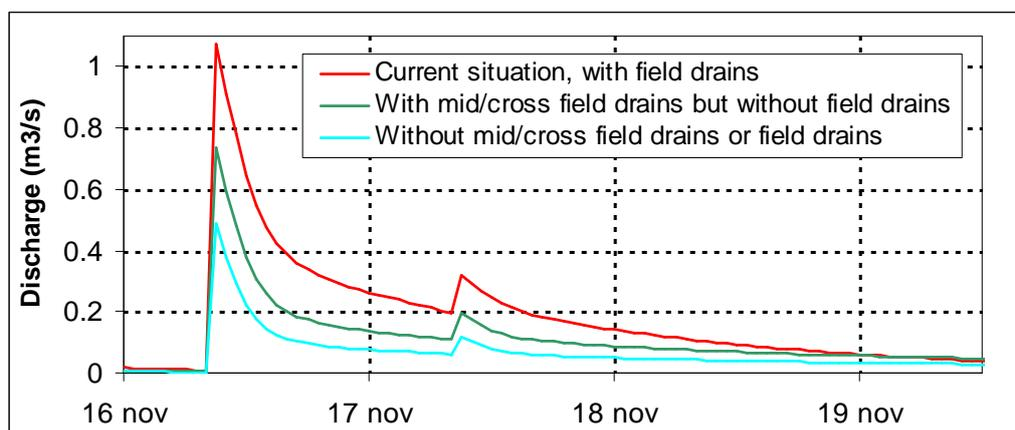
Figure 6 Modelled discharge following a 100 mm rain event with a typical return time of 1 year (followed by a smaller event), from 2 compartments as shown in Figure 7. According to model results, not having any field drainage would reduce peak discharge by more than 50%. Removing field drains but not mid/cross field drains could reduce peak discharge by 30%.
