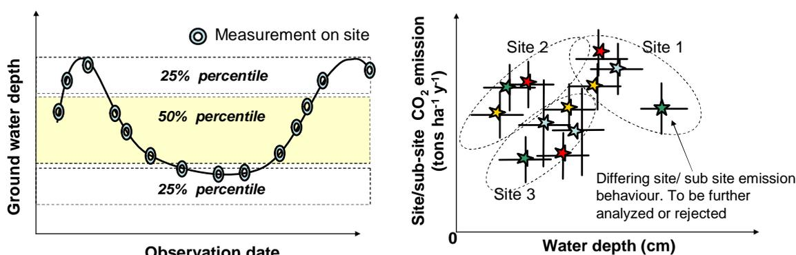
Figure 10 Schematic outline of data selection for analysis describing typical hydrological conditions during the observation period (left), and plot of emissions in the typical hydrological conditions on sites (right).
