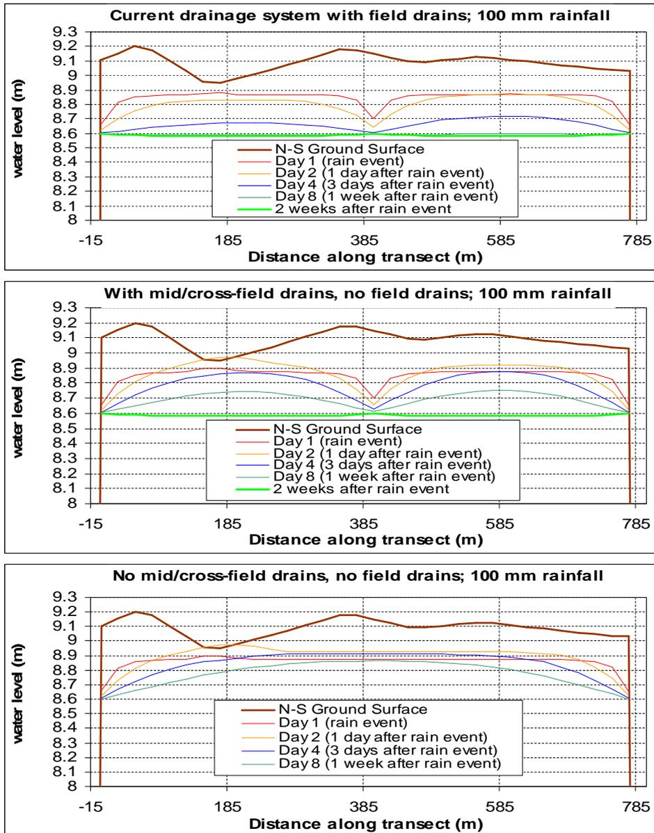
Figure 7 Modelled effectiveness of field drainage in discharging a 1-year rainfall event (100 mm of rainfall). It was assumed that the water table was at the upper range of the management target zone, i.e. 0.5m below the peat surface, at the start of the event. The following is observed:
