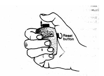
Figure 3: Tally counter used for accurately counting waterbird flocks.
