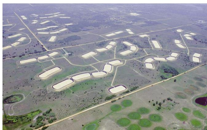
Figure 9 Rapid infiltration basins, Orlando, Florida (USGS)
