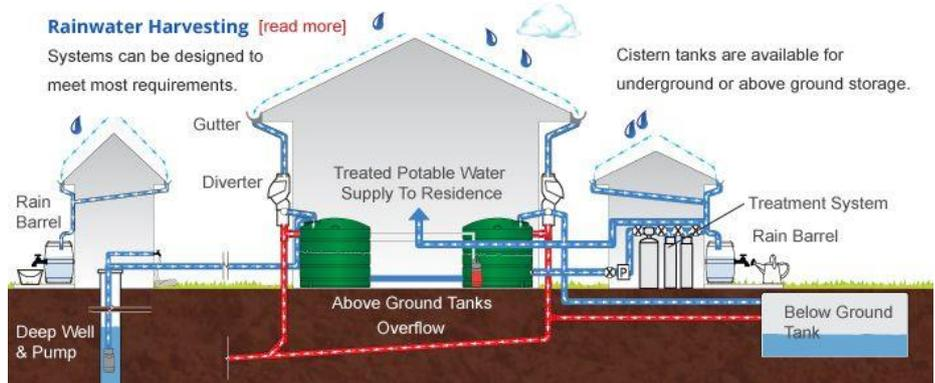
Figure 7 Rainwater Harvesting (Greenhouse engineering)
