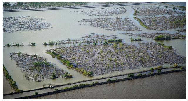
**Plate 18.** Pond dikes are disconnecting the tidal inundation of natural mangroves in the process of converting mangroves to fishponds in the Pampanga Delta, December 2016. Photo: Ivan Sarenas.
