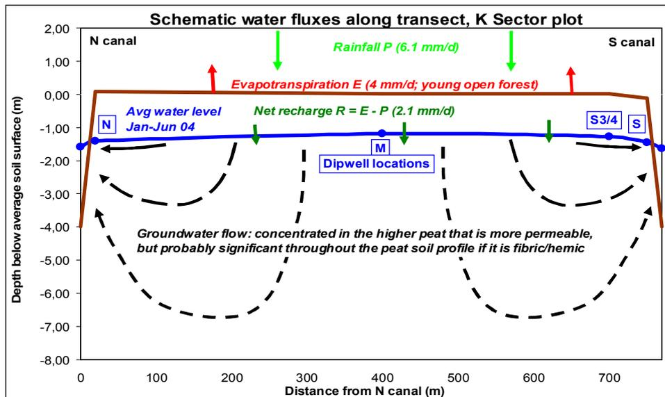
Figure 10 Schematization of water fluxes between parallel canals in a plantation. Note the near-flat shape of the average groundwater table, indicating rapid groundwater discharge due to high hydraulic conductivity of the peat. Hydraulic conductivity, and therefore water loss to groundwater, will be greatest in the deepest and least decomposed peat, i.e. further away from rivers.
