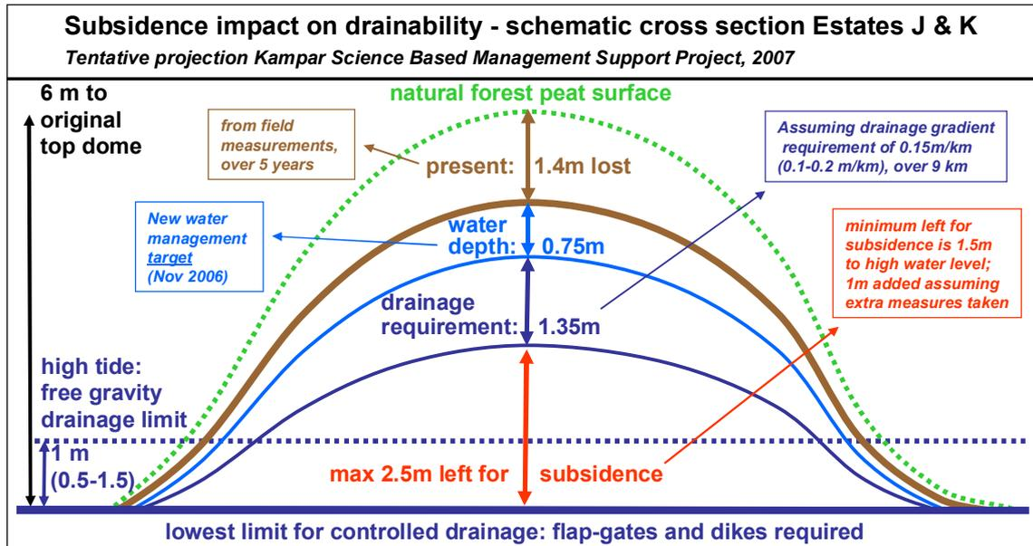
Figure 14 Subsidence impacts on drainability in schematic cross section through Estates J & K (in Pelalawan).
