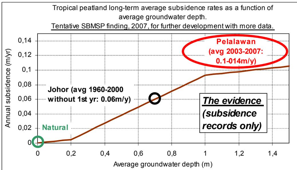
Figure 13 Tentative subsidence–water depth curve now applied in the Kampar SBMSP. Note that this applies to average subsidence over 50 years of drainage. The very high subsidence rate observed at Pelalawan plantations in recent years applies to the early years after drainage is implemented, and are the result of drainage to 1.2m water depth on average over this period; this rate will be reduced in coming years.
