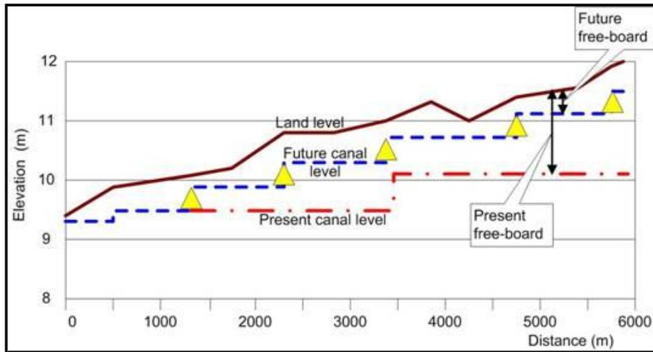
Figure 4 Schematic drawing of a cascade of dams to bring up water levels in the Madukoro Bawah Pilot area. Yellow triangles indicate planned dam locations.
