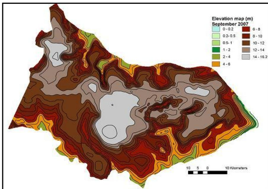
Figure 11 Kampar SBMS Project elevation map for the situation prior to drainage (2000), the basis for strategy assessments.
