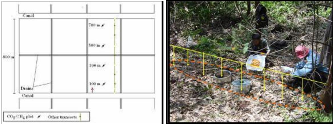
Figure 12 Schematic setup for soil C-gas ( $\text{CO}_2$  and  $\text{CH}_4$ ) emission measurements in drained acacia plantations, showing sampling locations across plantation compartments (left) and between trees (right). The sampling scheme is set up to A) distinguish between emissions resulting from decomposition and root respiration, and B) relate decomposition emissions to water depths.
