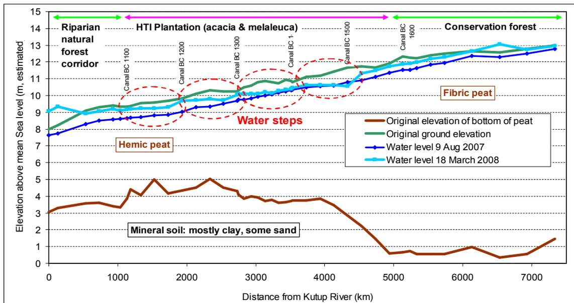
Figure 5 Water depth in dipwells and canals along transect in Madukoro Bawah Pilot Area. Water table fluctuations for this area are shown in Figure 2.
