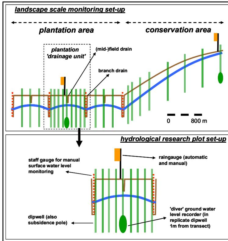
Figure 9 Schematized set-up of hydrometeorological monitoring transects within pilot areas.
