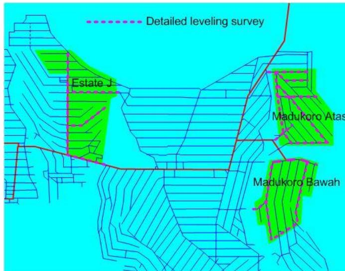
Figure 3 Pilot Areas within APRIL acacia plantations, and requirements for detailed elevation levelling. Conservation areas upslope from each pilot plantation area are included in the study.
